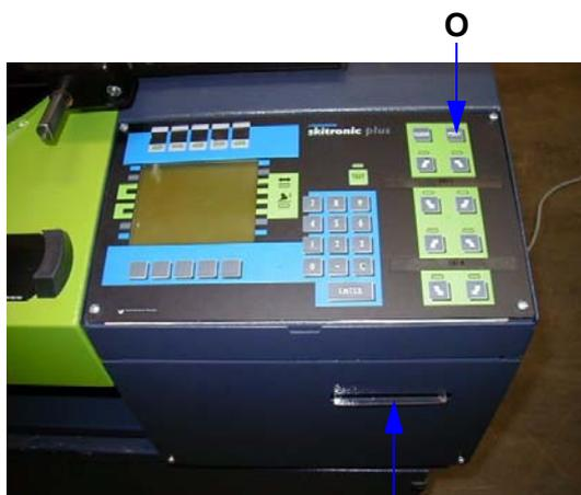
If all adjustments are correct for the left and right ski (the lamps for the corresponding releases must light (pos.2 and 3) a ticket is then entered into the front of the unit (1) and by means of the printing key (O) the printing process commences.
