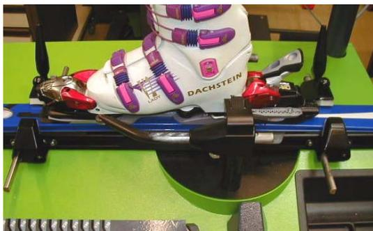
• The skis are placed in the center of the base unit (see the table, left) and if possible the two laterally mobile ski tighteners should be tightened close to the bindings in order that the skis should not be flexed unduly.
