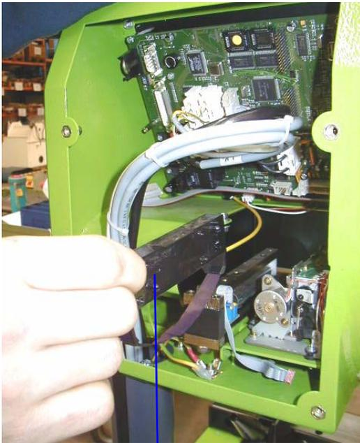
If the print-out on the card cannot be read easily the colour ribbon must be changed (1).
