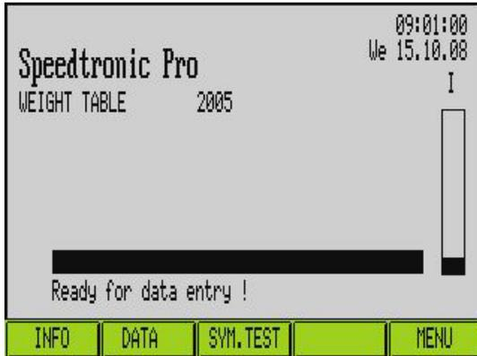
If the basic menu is visible in the display, you can start to enter the skier data by pressing the visual buttons.
