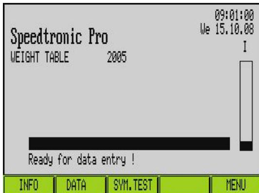
An inspection bar is located on the main screen of the corresponding selected method.
