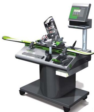
The corresponding data of the skier are entered into the device using the selection fields on the touchscreen display or the binding ticket; the installed computer then determines the release torques and presettings conforming to standards of each binding and then shows them on the display.
