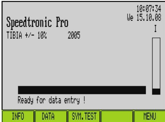
If the basic menu is visible in the display, you can start entering the skier data by pressing the visual buttons.
