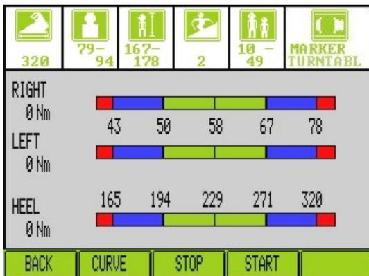
The boot is moved once to the left and once to the right until the maximum value has been exceeded. If the left-hand and right-hand maximum values are within the limited testing range, the procedure is stopped and the following screen is displayed.
