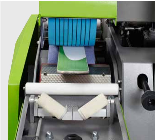
Centering unit supports custom racing structures
